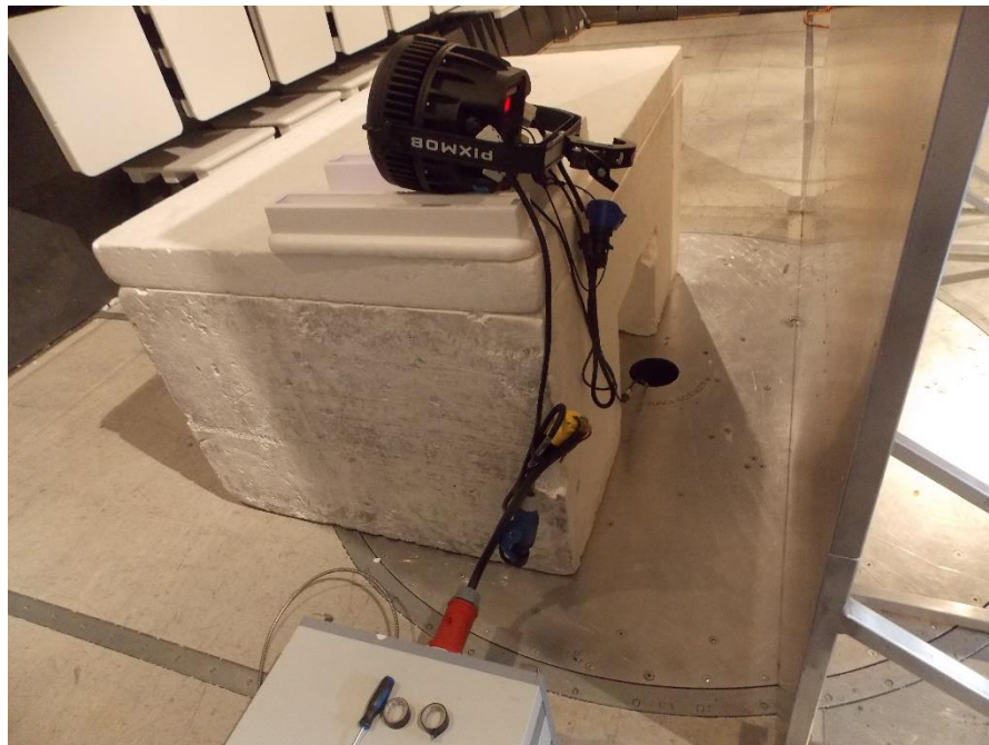
Figure 8.2-4: Conducted emissions – from AC mains power ports setup photo
