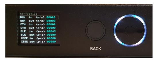
This screen indicates all the valid inputs and outputs in packets/seconds. This is useful for troubleshooting.
