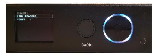
1. LINK BEACONS: Press on the Navigation Button to link all the Beacons that are in the Hub range. The LINK BEACONS line will turn red. The number of linked Beacons will appear on the COUNT line. Press again on the Navigation Button to stop linking Beacons. The linked Beacons will still be linked until the Hub is powered down.
