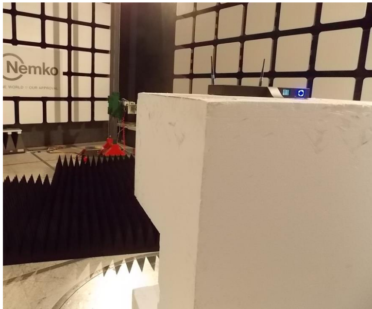
Figure 8.4-16: Radiated spurious (out-of-band) emissions setup photo – above 1 GHz
