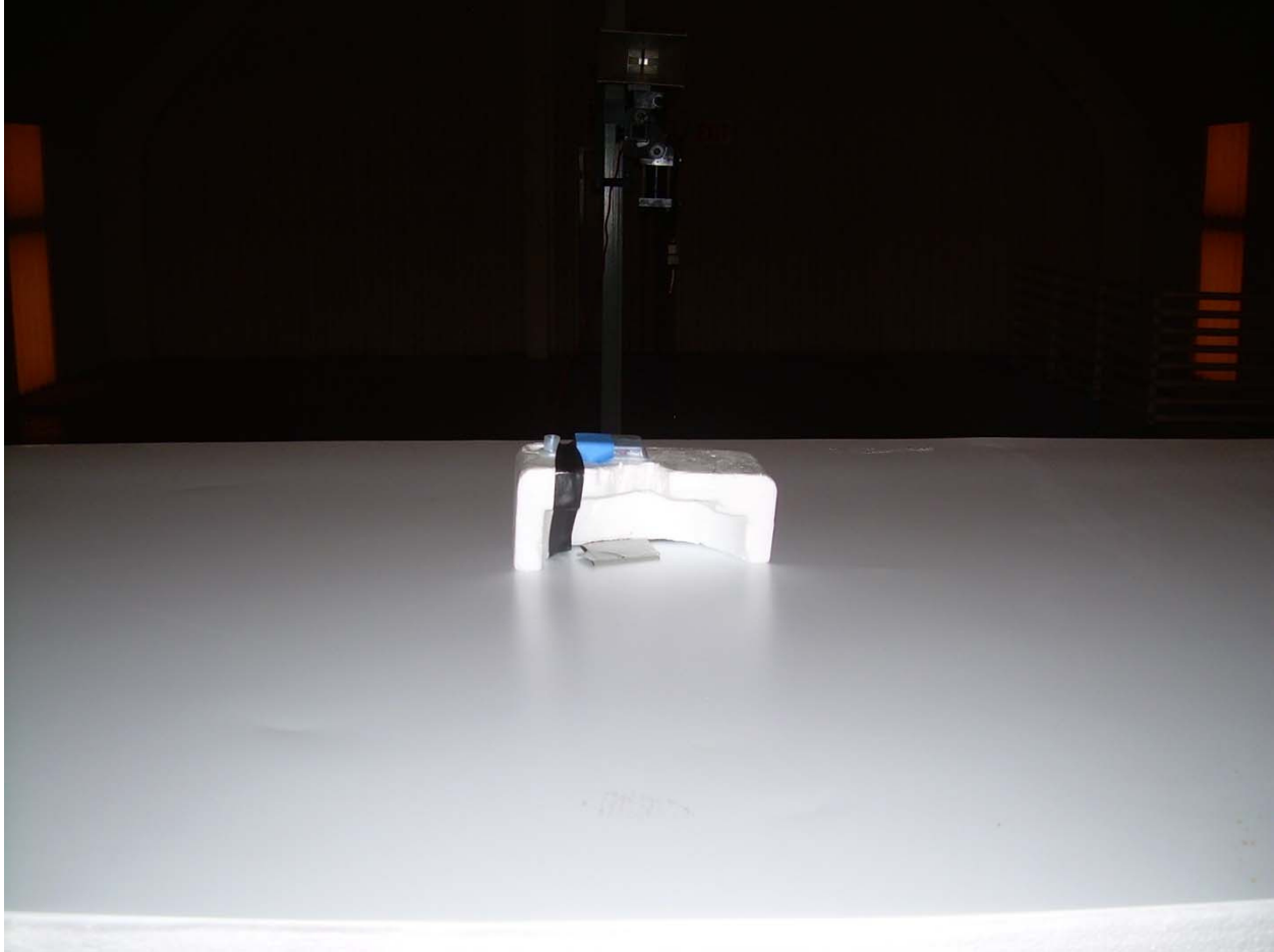
Photograph 3 – Back View Radiated Emissions – Above 1000 MHz Range – EUT Flat
