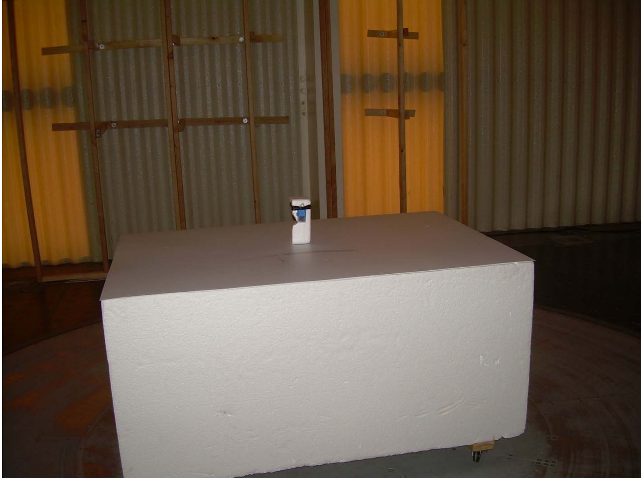
Photograph 1 – Front View Radiated Emissions – 9 kHz to 1000 MHz Range – EUT Vertical
