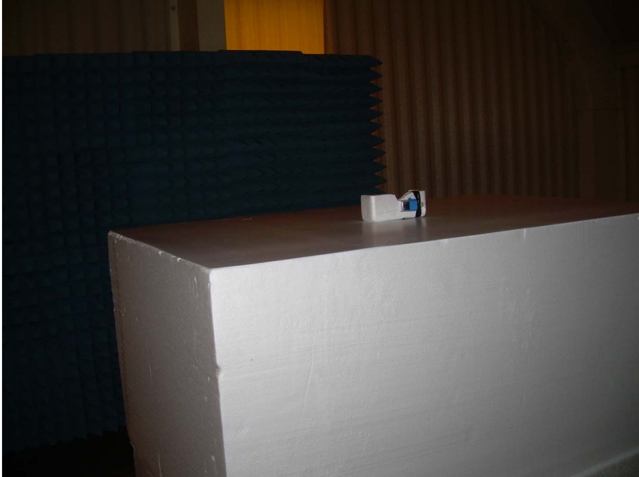
Photograph 2 – Front View Radiated Emissions – Above 1000 MHz Range – EUT On Edge
