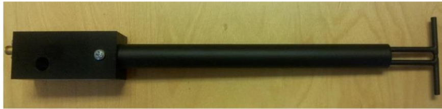
Figure 1 – MVG COMOSAR Validation Dipole
