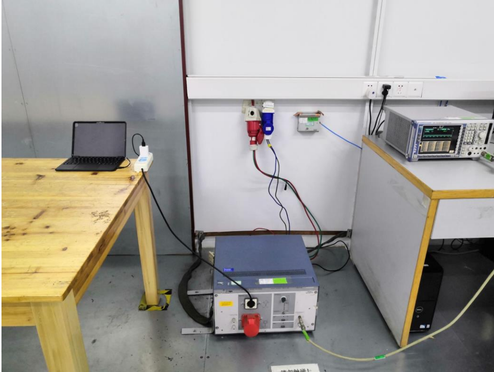
CONDUCTED TEST SETUP
