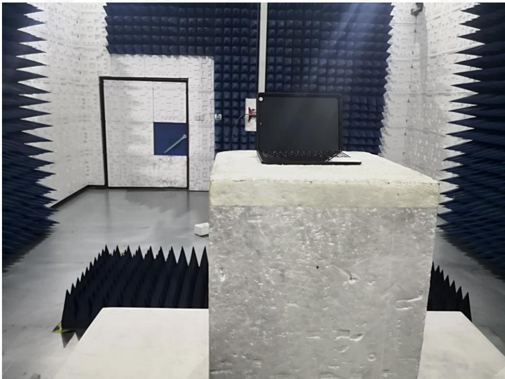
FCC RADIATED EMISSION TEST SETUP ABOVE 1GHZ
