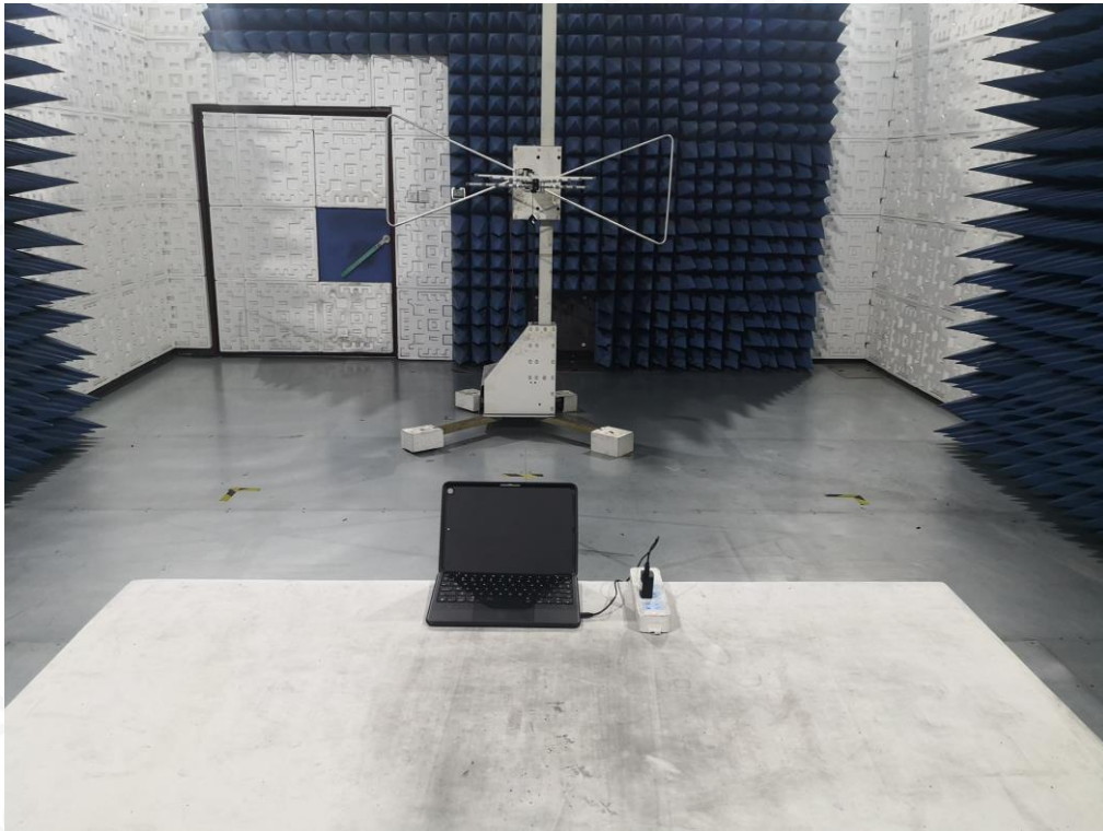
FCC RADIATED EMISSION TEST SETUP ABOVE 1GHZ
