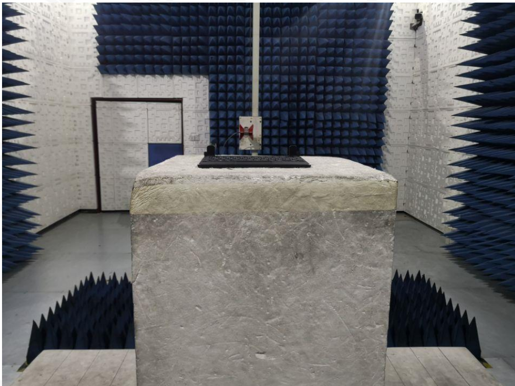
FCC RADIATED EMISSION TEST SETUP ABOVE 1GHZ
