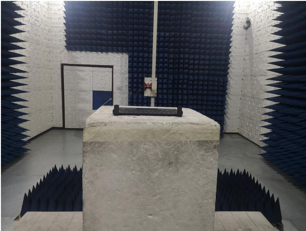
FCC RADIATED EMISSION TEST SETUP ABOVE 1GHZ
