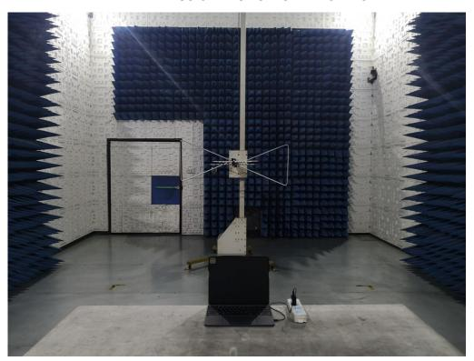
RADIATED EMISSION TEST SETUP ABOVE 1GHZ
