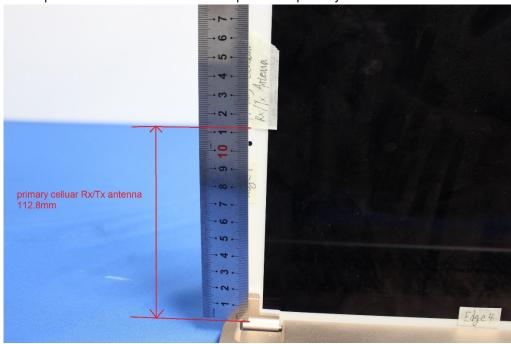
The separation distances between the Ipad Pro's WiFi/BT antenna to the upper edge of the EUT
