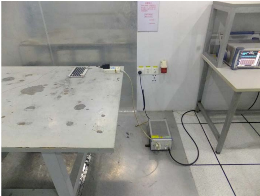
1 Photo of Power Line Conducted Emission Measurement
