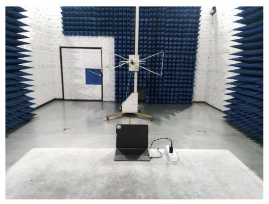
RADIATED EMISSION TEST SETUP ABOVE 1GHZ
