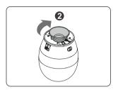
Fasten the adaptor by turning it gently in the clockwise direction.
