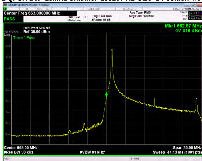
Band71 QPSK BW=15MHz Channel=133197 RB Size=1 Position=#Max Extended
