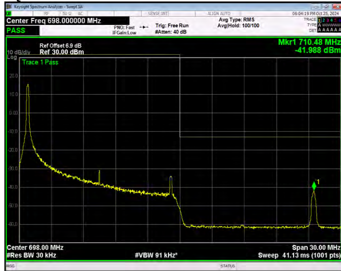
Band71 QPSK BW=15MHz Channel=133397 RB Size=#Max Extended
