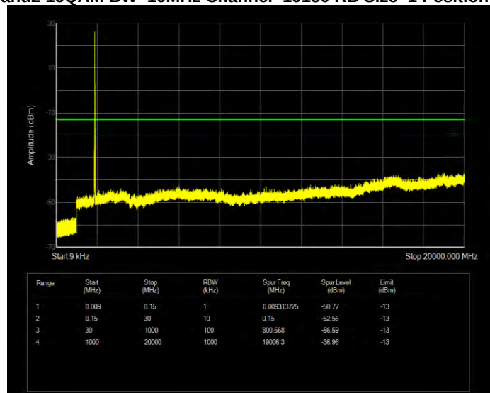
Band2 16QAM BW=15MHz Channel=18675 RB Size=1 Position=#0
