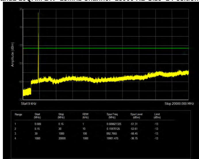
Band2 16QAM BW=15MHz Channel=19125 RB Size=1 Position=#0
