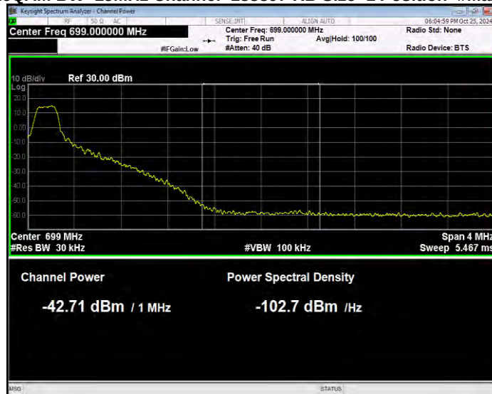
Band71 16QAM BW=15MHz Channel=133397 RB Size=1 Position=#Max Normal
