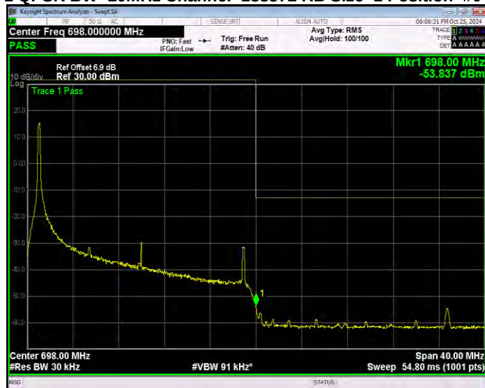
Band71 QPSK BW=20MHz Channel=133372 RB Size=1 Position=#Max Extended
