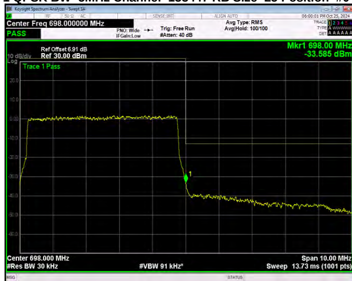
Band71 QPSK BW=5MHz Channel=133447 RB Size=25 Position=#0 Normal
