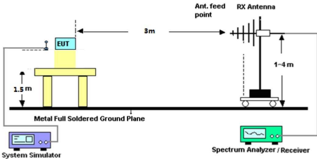
For radiated test from above 1GHz
