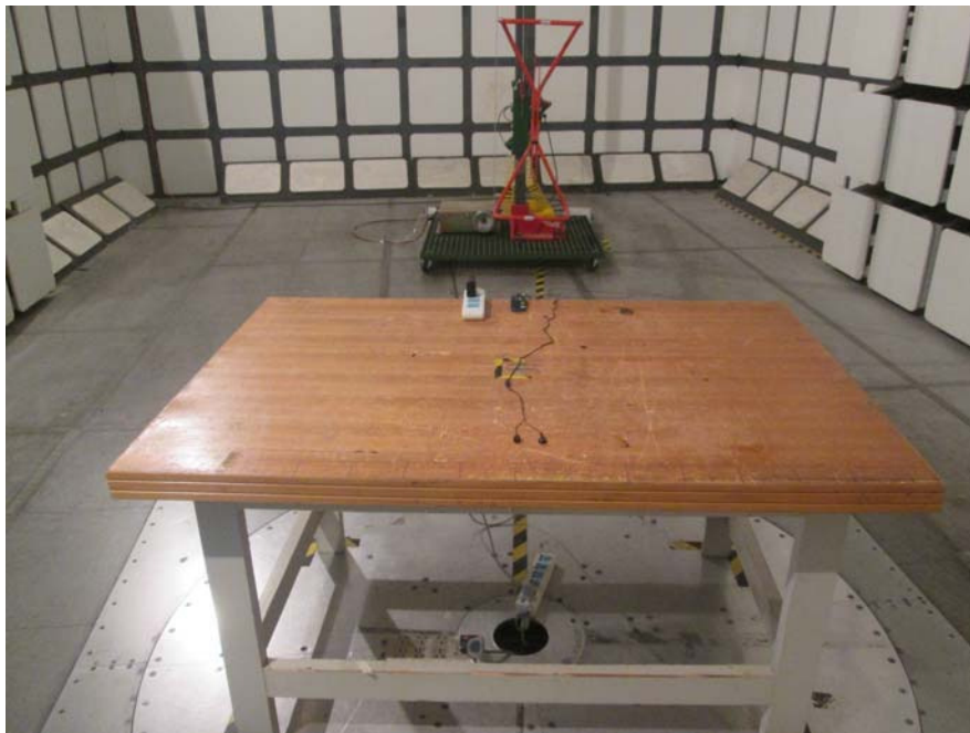
Radiated Emissions Front View (Below 1 GHz)
