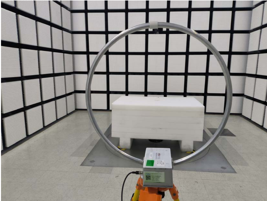
Radiated Emission 9kHz-30MHz View-Perpendicular
