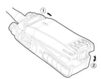
To remove the battery, turn off the radio first. Then slide the battery latch upwards to unlock the battery.
