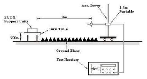
The radiated emissions were performed in the 3 meters chamber test site, using the setup accordance with the ANSI C63.4-2014. The specification used was with the FCC Part 15 B Class B limits.
