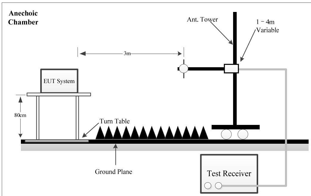
The radiated emission tests below 1GHz were performed at the 3 meters distance, above 1GHz were performed at the 3 meters Chamber B, using the setup accordance with the ANSI C63.4-2014. The specification used was the FCC Part 15B Class B limits.
