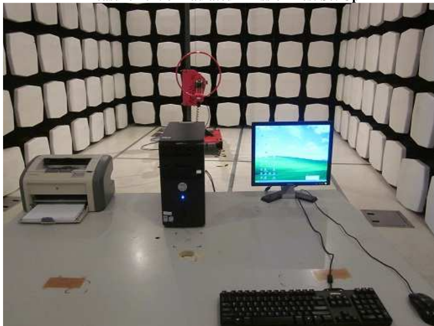
Measurement of Radiated Emission Test Set Up
