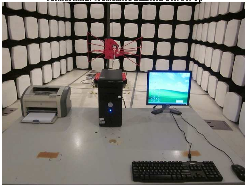
Measurement of Radiated Emission Test Set Up
