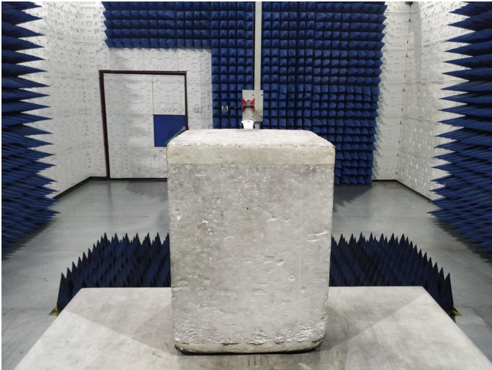
RADIATED EMISSION TEST SETUP ABOVE 1GHZ
