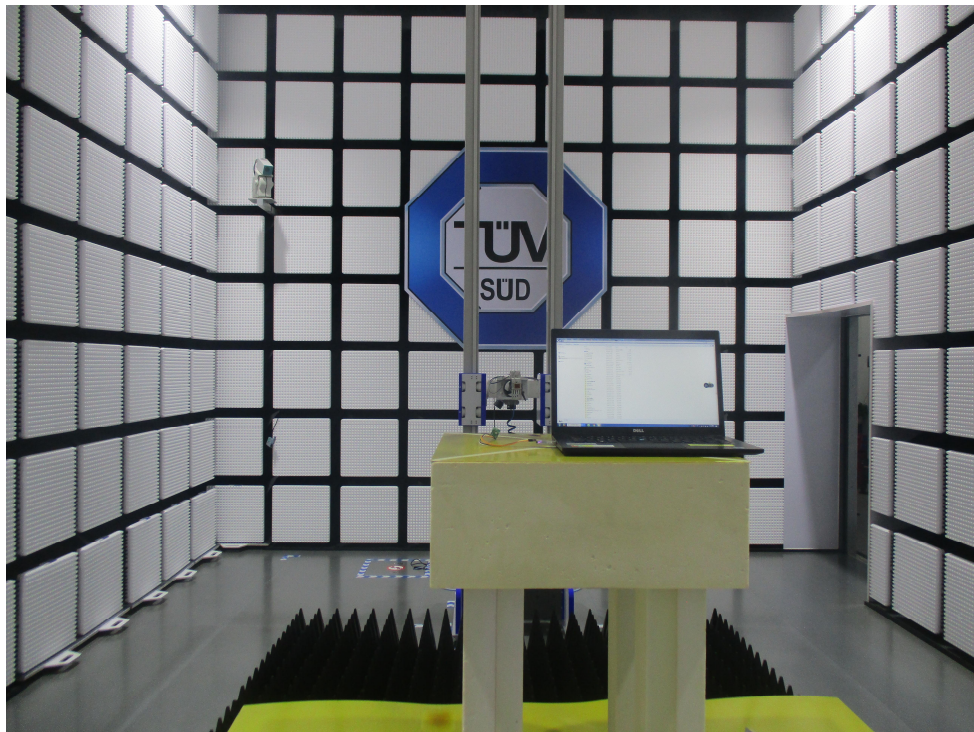
Radiated Emission Test below 18GHz-40GHz
