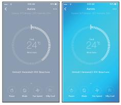
(3) Thus, user can control air conditioners on/off status, operation mode, temperature, fan speed and so on.
