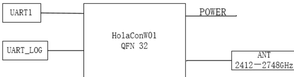
figure 1. Module System Block Diagram
