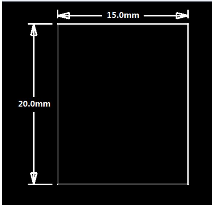
The size of the module as shown above , length:20.0mm, width:15.0mm, thickness 1.0mm (error +/- 0.1mm)
