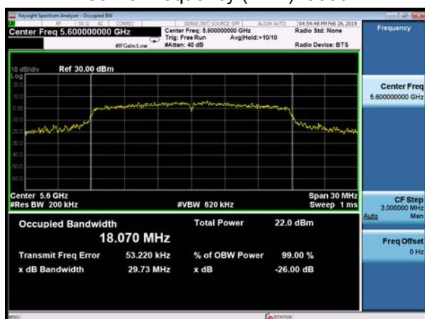
U-NII-2C, 802.11n HT20 Carrier frequency (MHz): 5700
