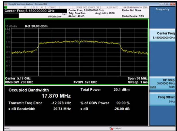
U-NII-1, 802.11n HT20 Carrier frequency (MHz): 5200
