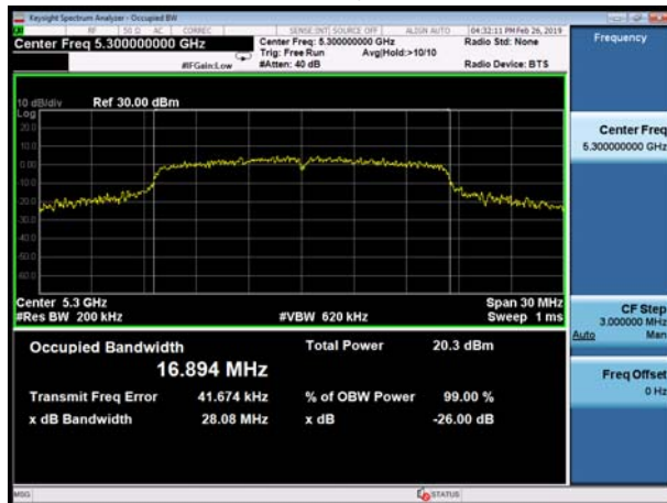
U-NII-2A, 802.11a Carrier frequency (MHz): 5320
