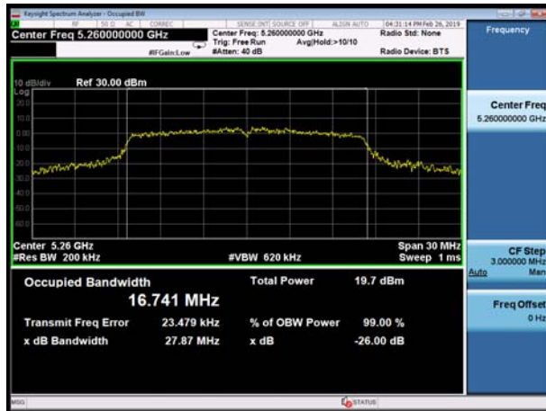
U-NII-2A, 802.11a Carrier frequency (MHz): 5300
