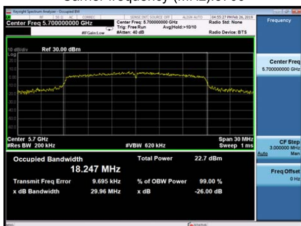
U-NII-2C, 802.11n HT20 Carrier frequency (MHz): 5700
