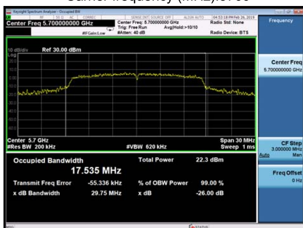
U-NII-2C, 802.11a Carrier frequency (MHz): 5700
