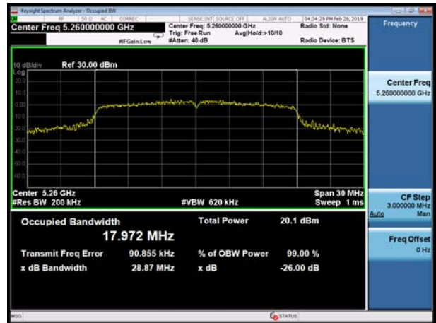
U-NII-2A, 802.11n HT20 Carrier frequency (MHz): 5300
