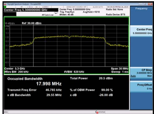
U-NII-2A, 802.11n HT20 Carrier frequency (MHz): 5320
