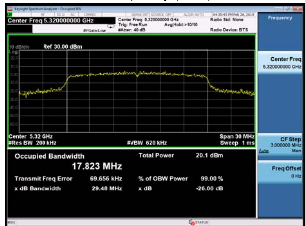
U-NII-2A, 802.11n HT20 Carrier frequency (MHz): 5320
