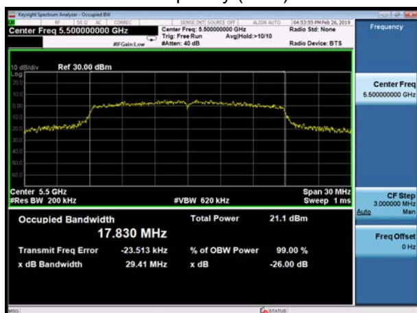
U-NII-2C, 802.11n HT20 Carrier frequency (MHz): 5600
