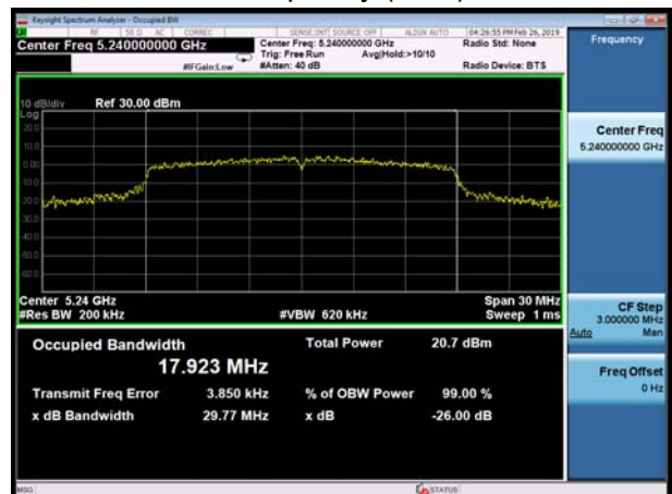
U-NII-1, 802.11n HT20 Carrier frequency (MHz): 5240
