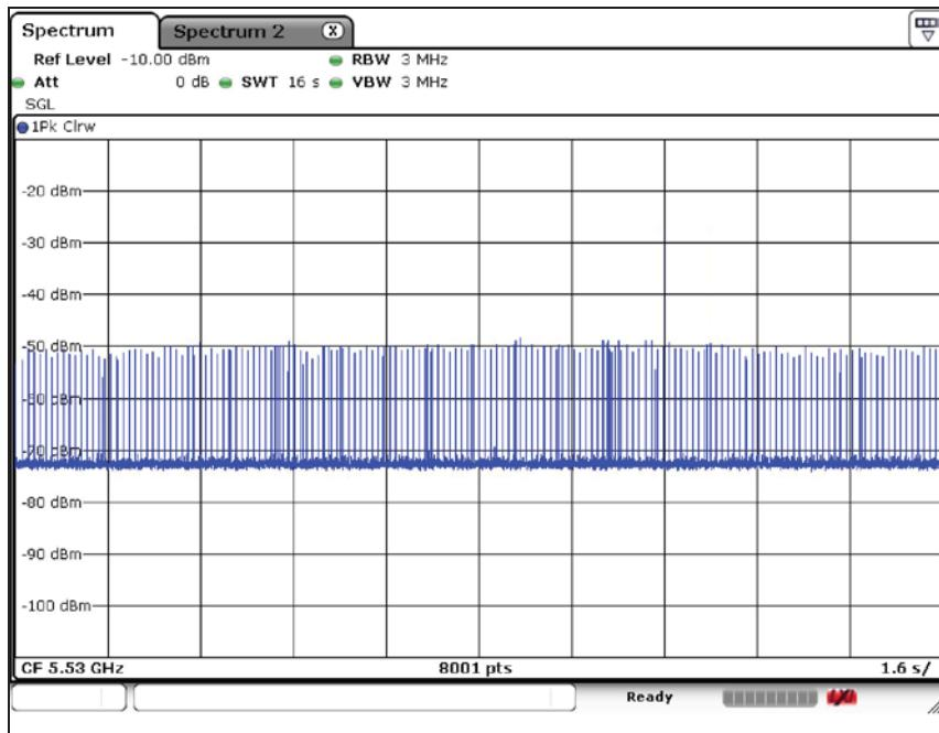
**Channel Loading****11ac\_VHT80****5 290 MHz**
