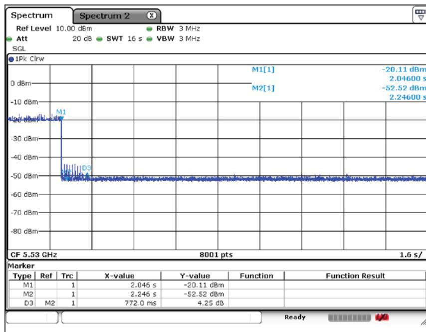
**Plot of Non-occupancy period****11ac\_VHT80****5 290 MHz**
