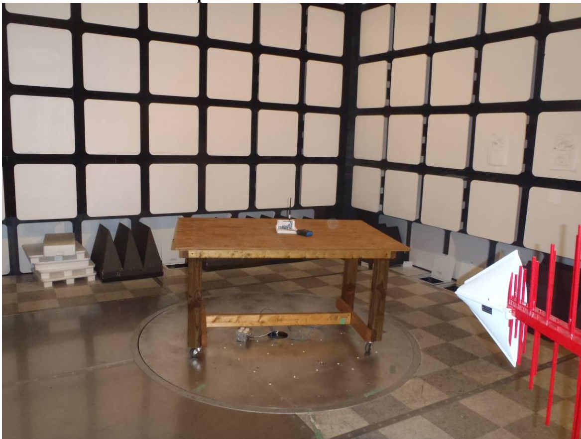
Radiated Emission Test Setup Photo#1:
