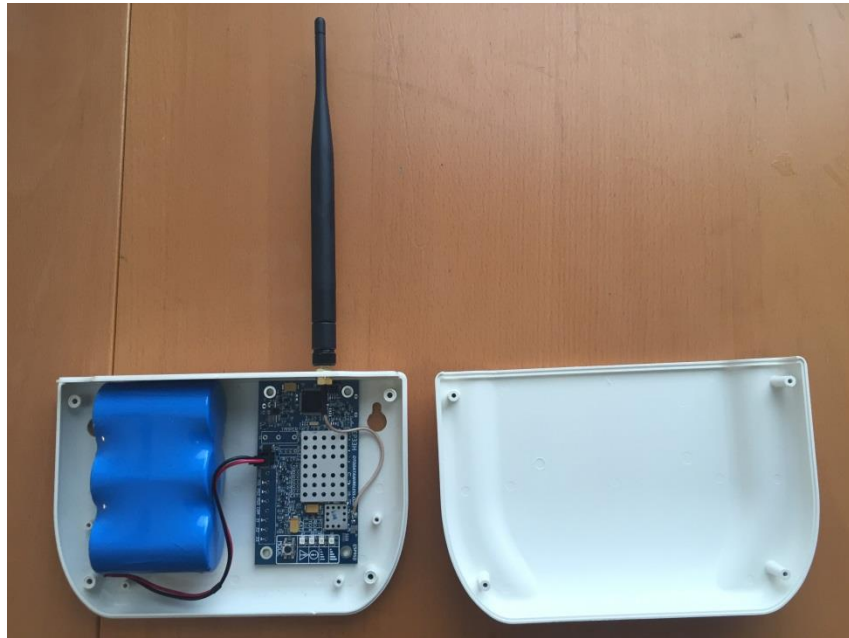
C005 Top inside with marketed SMA-RP connector
