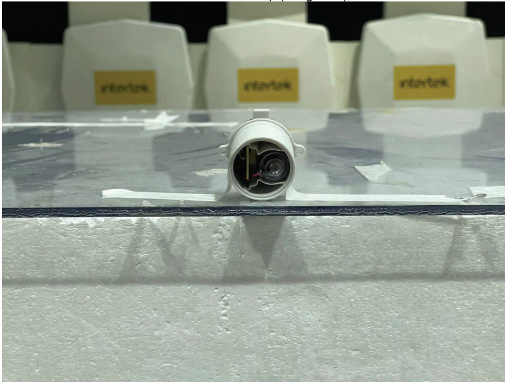
Radiated Emission Test Setup (Long Side), 1-13 GHz
