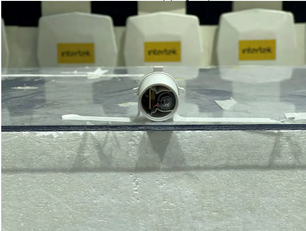
Radiated Emission Test Setup (Long Side), 1-13 GHz
