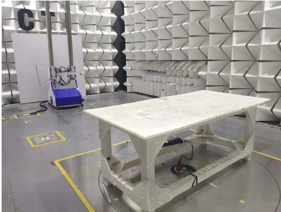
Radiated spurious emission Test Setup-1(Below 1GHz)
