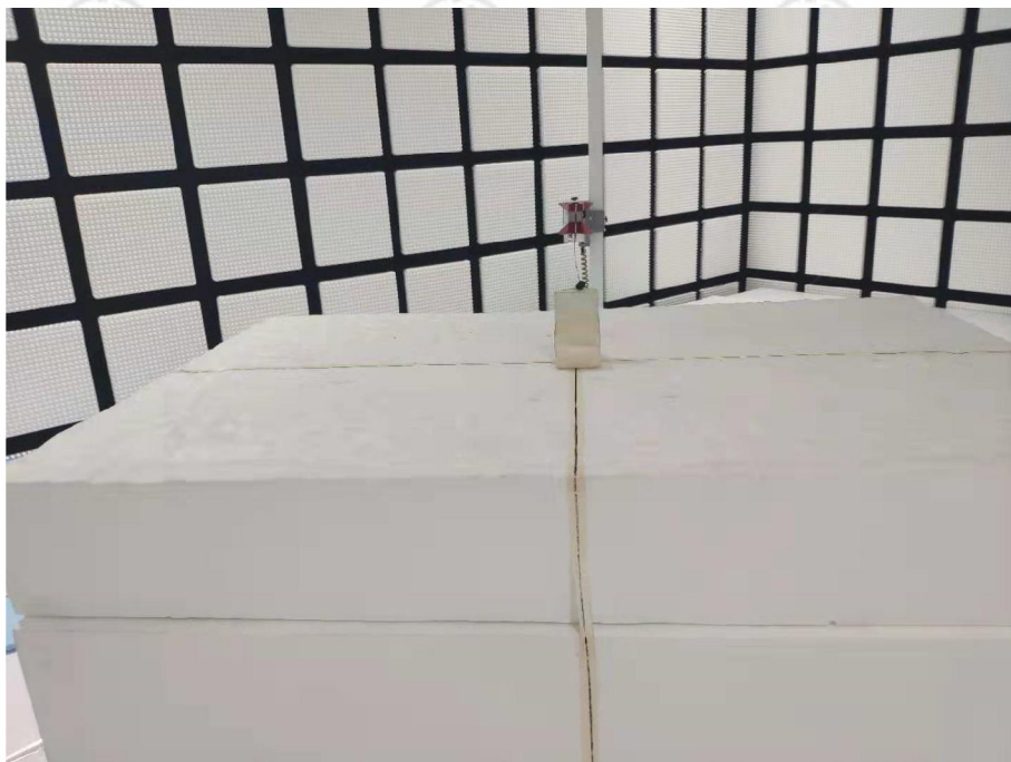
Radiated spurious emission Test Setup-2(Above 1GHz)
