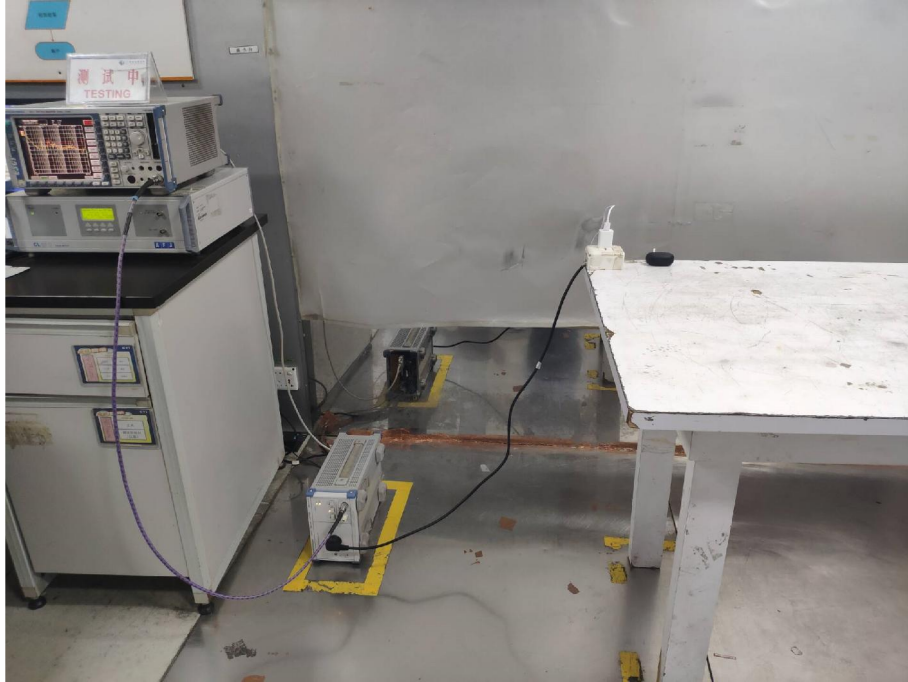
Conducted Emissions Test Setup
