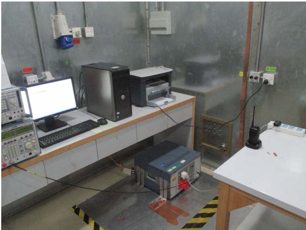
CONDUCTED EMISSION TEST SETUP
