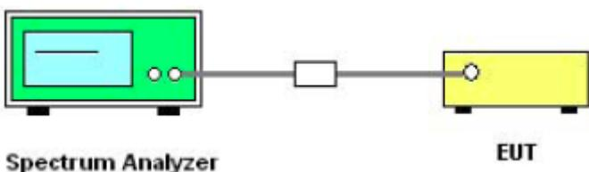
The EUT which is powered by the Battery, is coupled to the Spectrum Analyzer; the RF load attached to the EUT antenna terminal is 50Ohm; the path loss as the factor is calibrated to correct the reading. Make the measurement with the spectrum analyzer's resolution bandwidth(RBW) = 100 kHz. In order to make an accurate measurement, set the span greater than RBW.
