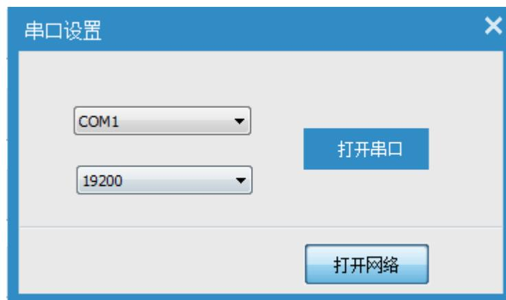
Select the right port and set the baud rate (default setting is 19200bps); and then click open serial port to enable the communication between serial port and fixture board.
