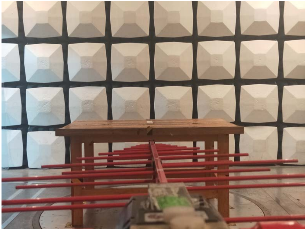
Radiated Emission Above 1GHz View
