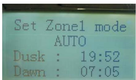
WHEN YOU CHOOSE "AUTO" MODE, AND ENTER TO EMIT THE RF SIGNAL "AUTO" TO RXS IN SOLO ZONE, RXS WILL BE ACT "AUTO". THE TIME OF "DUSK" AND "DAWN" IS CALCULATED AUTOMATICALLY BY MASTER. WHEN MASTER IS RUN BACK TO MAIN INTERFACE AND SHOWS "AUTO" ICON "●"
