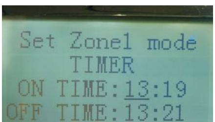
WHEN YOU CHOOSE "TIMER" MODE, SET THE TIME ON AND TIME OFF THAT YOU NEED, AND ENTER TO EMIT THE RF SIGNAL "TIMER" TO RXS IN SOLO ZONE, RXS WILL BE ACT "TIMER". MASTER IS RUN BACK TO MAIN INTERFACE AND SHOWS "TIMER" ICON "🕒"
