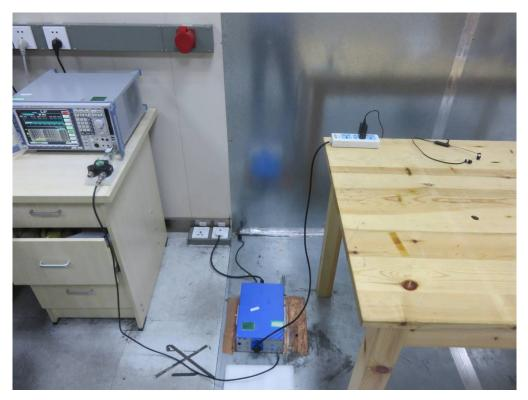
FCC RADIATED EMISSION TEST SETUP
