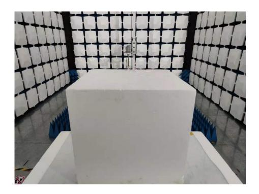
Blow 1GHz for radiated emission test setup
