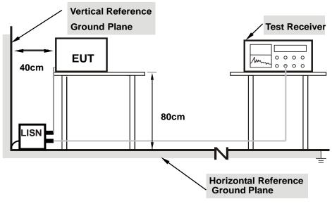
Note: 1.Support units were connected to second LISN. 2.Both of LISNs (AMN) are 80 cm from EUT and at least 80 from other units and other metal planes
