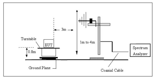
(C) Radiated Emission Test-Up Frequency Above 1GHz
