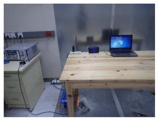
FCC RADIATED EMISSION TEST SETUP
