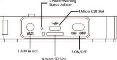
1. AUX in slot : insert 3.5mm audio cable , Press **M** button to "Aux in mode" work as the external speaker of audio source of PSP/MP4 Etc.
