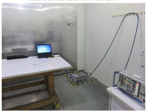
FCC RADIATED EMISSION TEST SETUP
