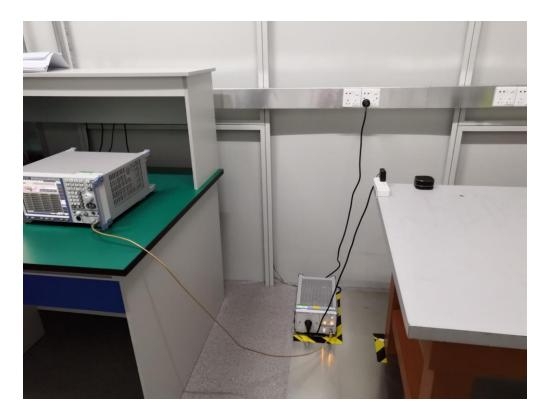
FCC RADIATED EMISSION TEST SETUP
