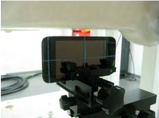
Fig.12 EUT right side to flat phantom
