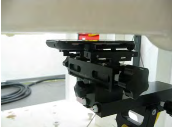
Fig.9 EUT front side to flat phantom
