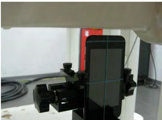
Fig.14 EUT top side to flat phantom
