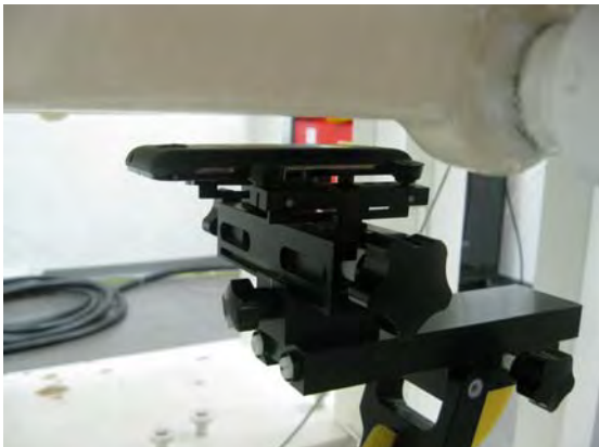
Fig.8 EUT back side to flat phantom
