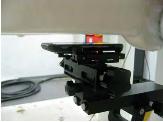
Fig.7 EUT front side to flat phantom
