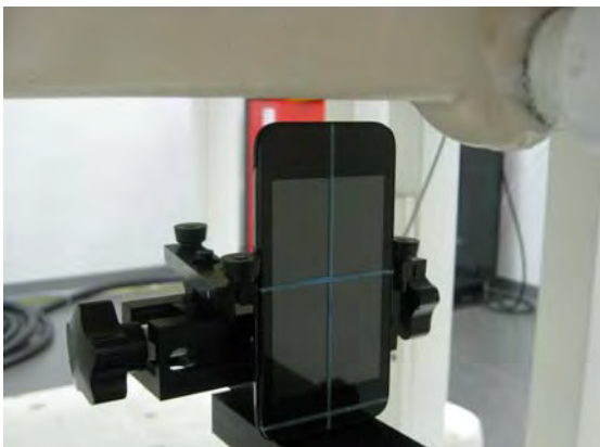
Fig.11 EUT bottom side to flat phantom
