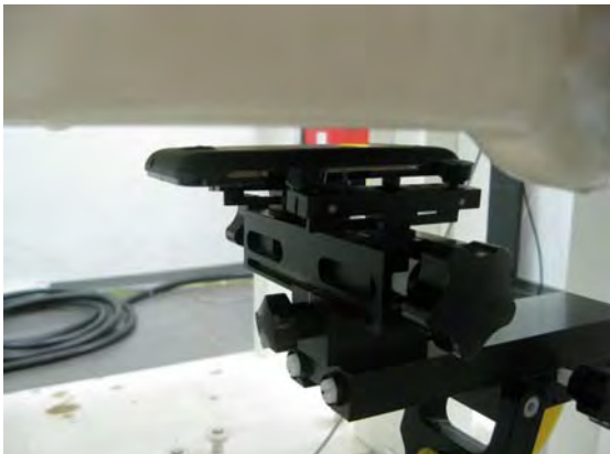
Fig.10 EUT back side to flat phantom
