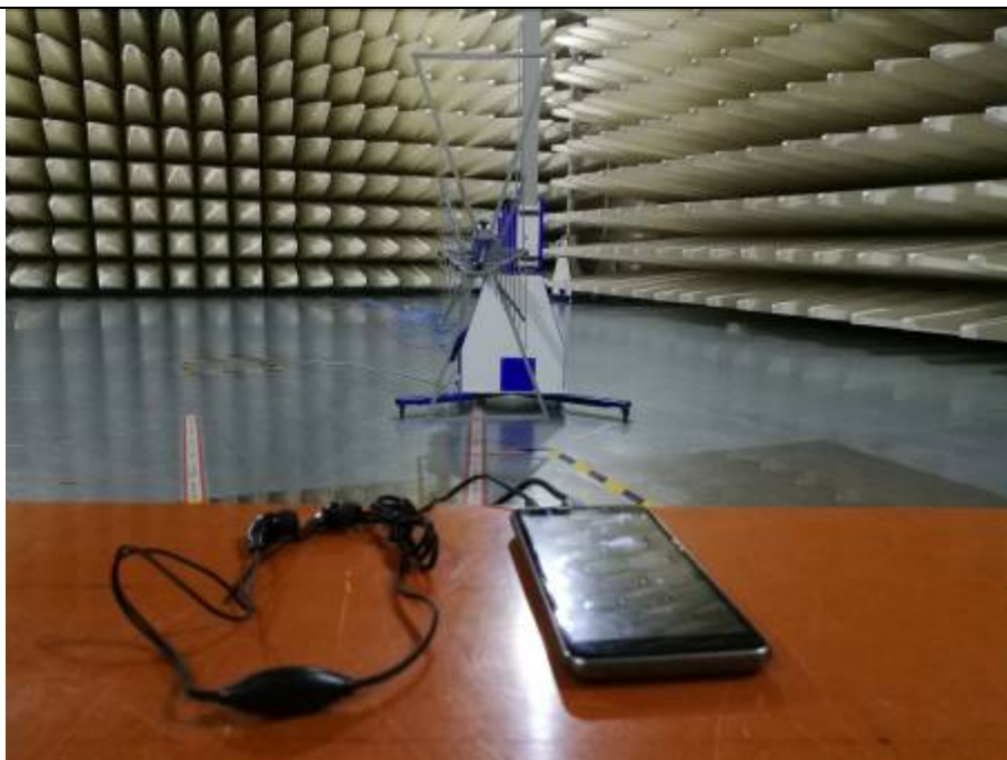
Spurious Radiated Emissions Test setup (30MHz~1GHz)
