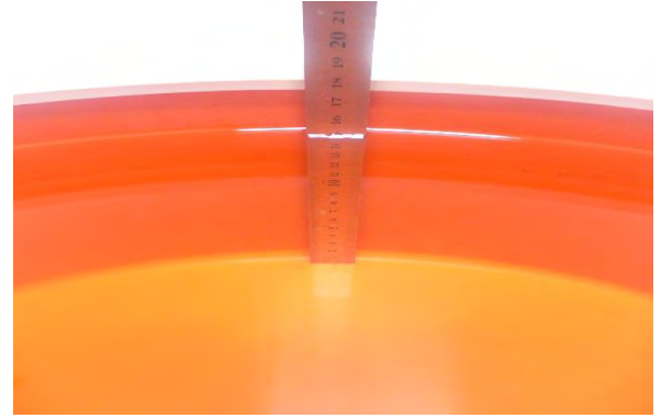
Photo 8: Tissue Simulant Liquid for Body 2450
