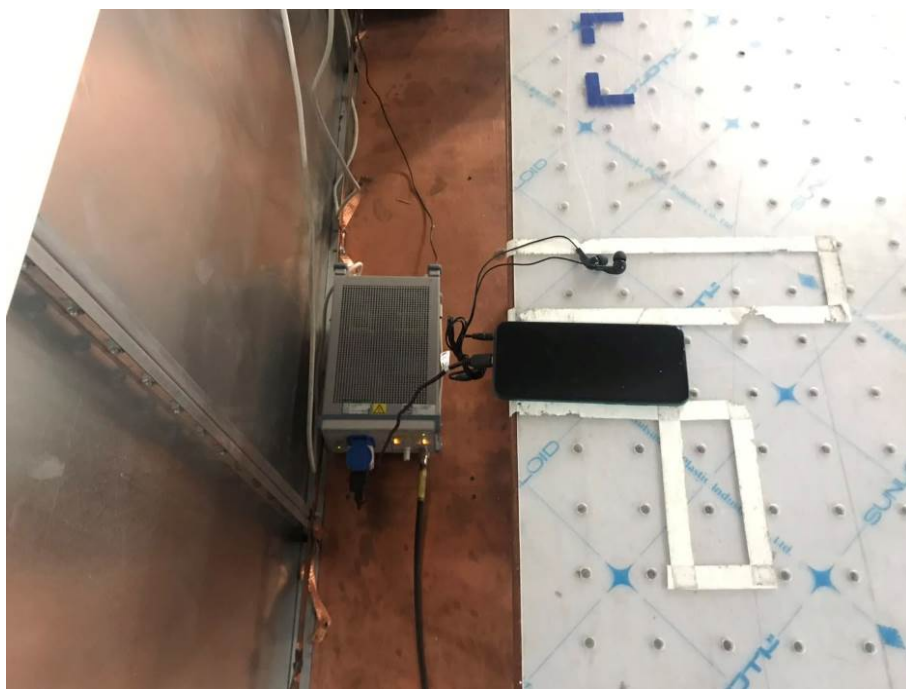
Conducted Emissions Test Setup (with charger)
