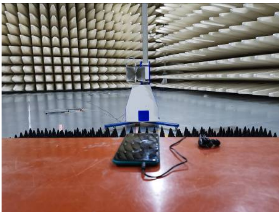
Radiated Emissions Test Setup (above1GHz)
