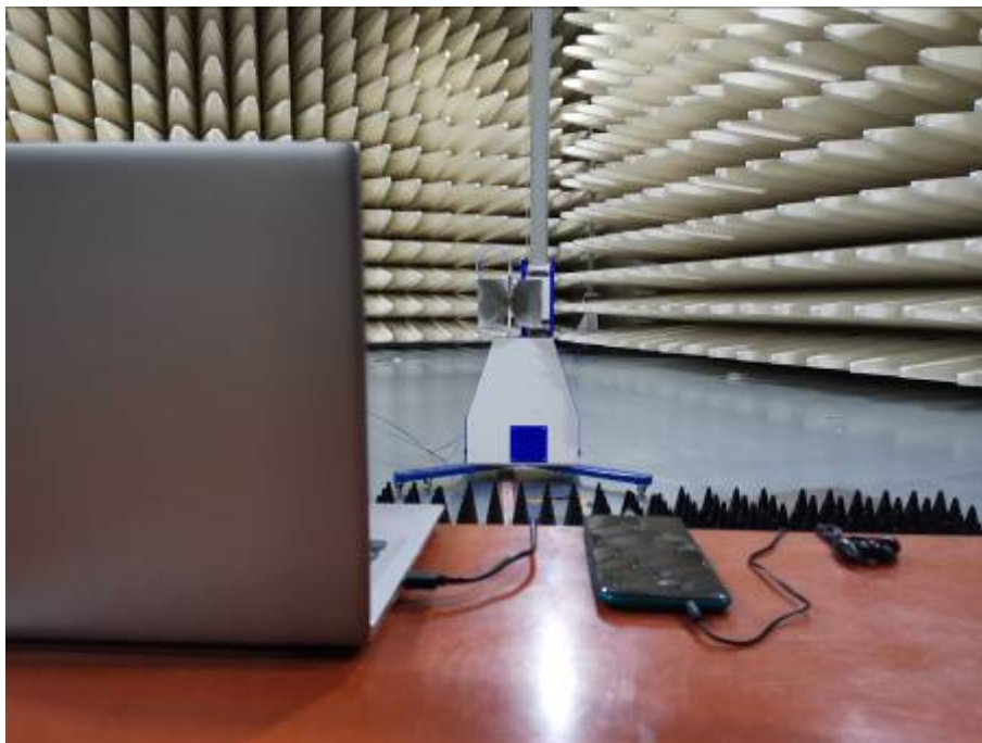
Radiated Emissions Test Setup (above 1GHz)
