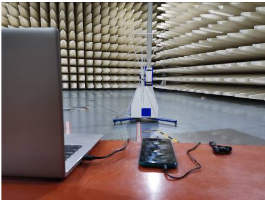
Radiated Emissions Test Setup (30-1000MHz)
