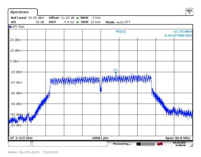
Carrier frequency (MHz): 2412 Channel No.1 Test Mode: 802.11g
