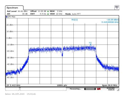
Carrier frequency (MHz): 2412 Channel No.1 Test Mode: 802.11n (HT20)
