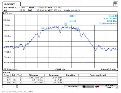
Carrier frequency (MHz): 2462 Channel No.:11 Test Mode: 802.11b
