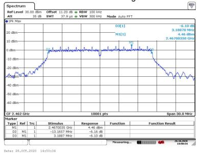
Carrier frequency (MHz): 2462 Channel No.:11 Test Mode: 802.11g
